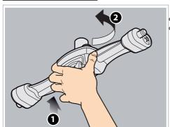
The impeller can be removed to make cleaning the oven cavity easier. Do this by pushing upward and unscrewing it counter-clockwise.
