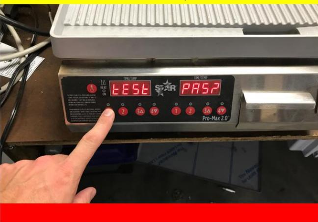
The timer will reset to 5:00 minutes, and start testing upper left platen.
