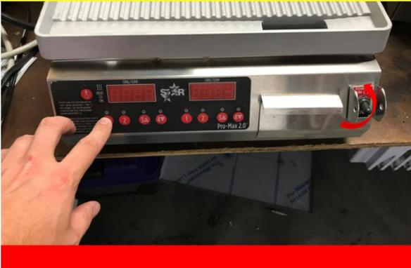
Unit will start 'TEST' mode and will start a 5:00 minute timer. The first test is always the bottom platen and the diagnostics will verify that the platen will increase 25°F within the 5 minutes.
